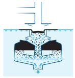
Deflection disks force the surface pollution and the water to the periphery. As the flow velocity drops, the surface pollution floats upwards while the water flows down through the outlet.
