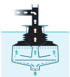
When the Surfcleaner has collected enough surface pollution the propeller reverses and, with the water acting as a piston, the surface pollution is discharged into an external container.
