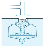
The propeller in the bottom creates negative pressure, causing the water and the surface pollution to flow into the Surfcleaner.
