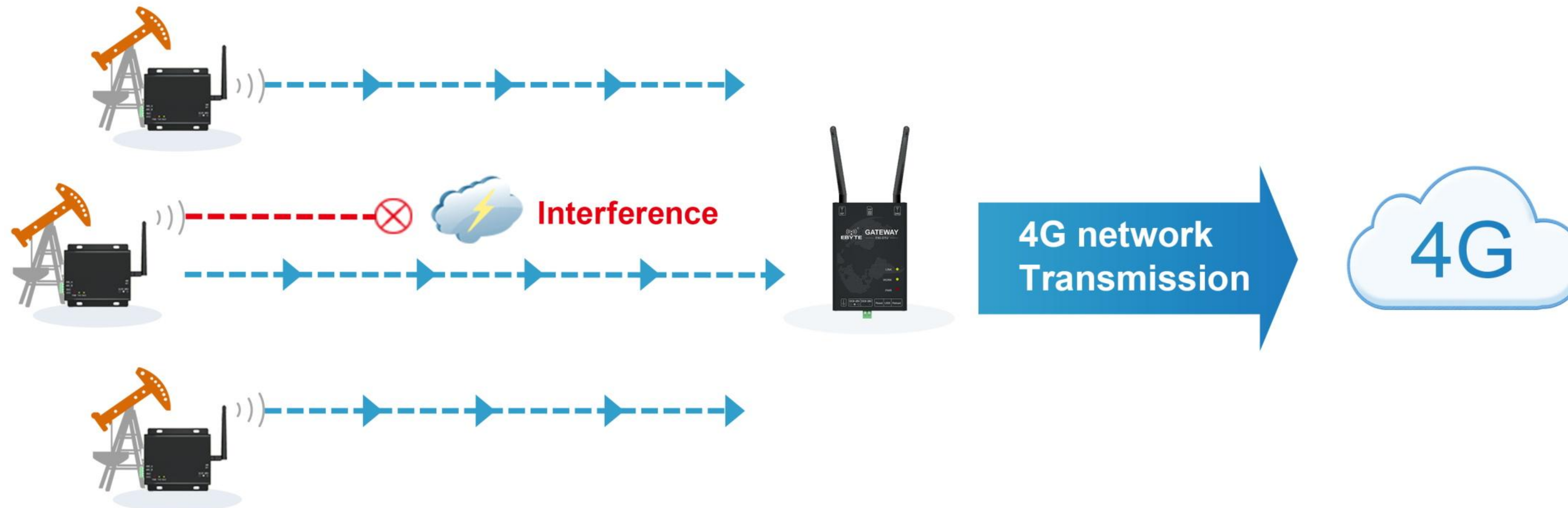
LoRa spread spectrum communication: anti-interference, longer transmission distance, and stable communication
